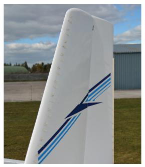
Left The vortex generators down the left side of the fin. In association with changes to the thrust line they resolved a serious handling issue resulting from a change of engine.
